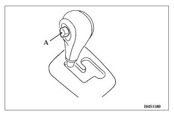
In the main gate, the selector lever has 4 positions and is equipped with a lock button (A) to prevent inadvertent selection of the wrong gear.
